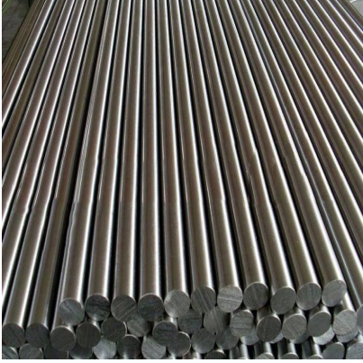
MS Bright Bar Rounds Dia 18.00mm
