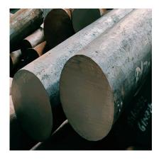
EN24 Forged Rounds in Annealed Condition â?? Ready for Machining & Heat Treatment
