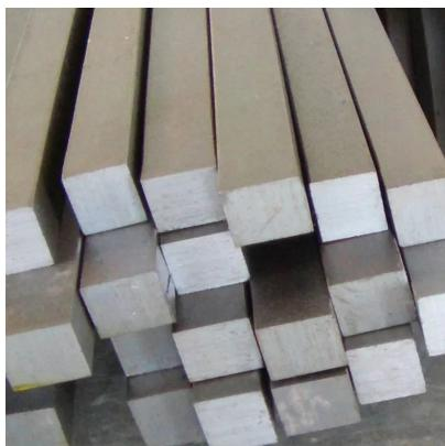
Mild Steel Square Bars (20â??52 MM) â?? Hot Rolled Black MS Squares | LC Commercial Steel
