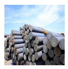
Mild Steel Round Bars (Dia 53â??65 MM) â?? Hot Rolled Black Rounds | LC Steel
