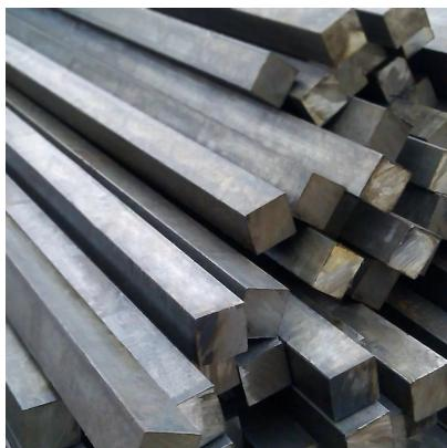
EN8 Hot Rolled Black Square Bars ?? 16mm to 150mm ?? Tough Medium Carbon Steel for Engineering Use
